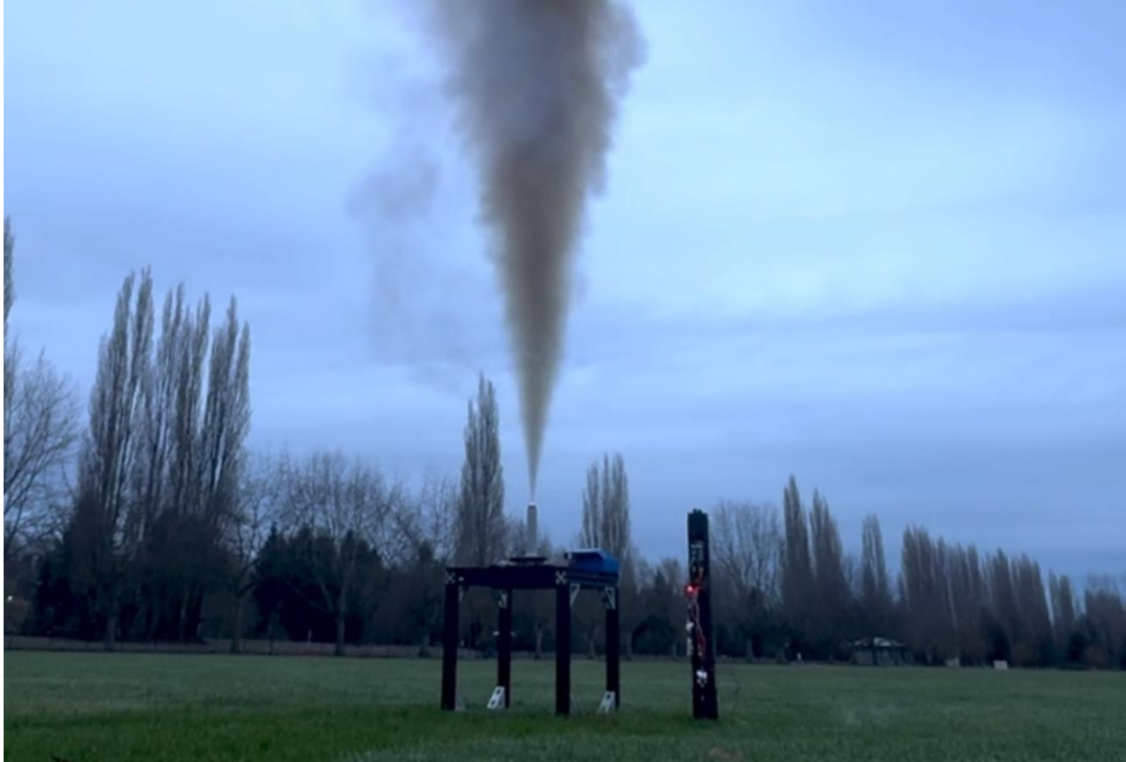
Figure 4: Thrust testing of the G33 SRM
